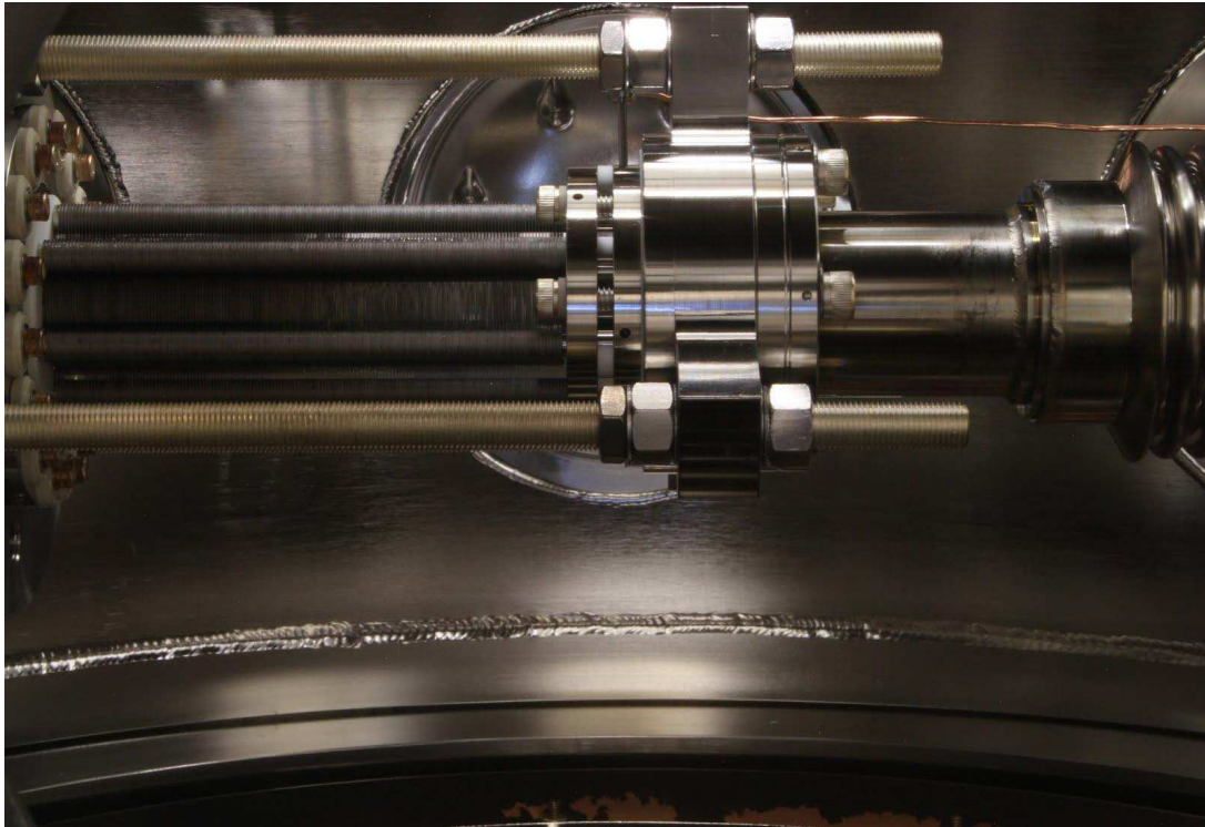
Figure 11 Side view of the funnel installed inside chamber B.
